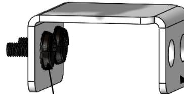
After assembly the M6 fixation apply glue on this surface to fix wall
