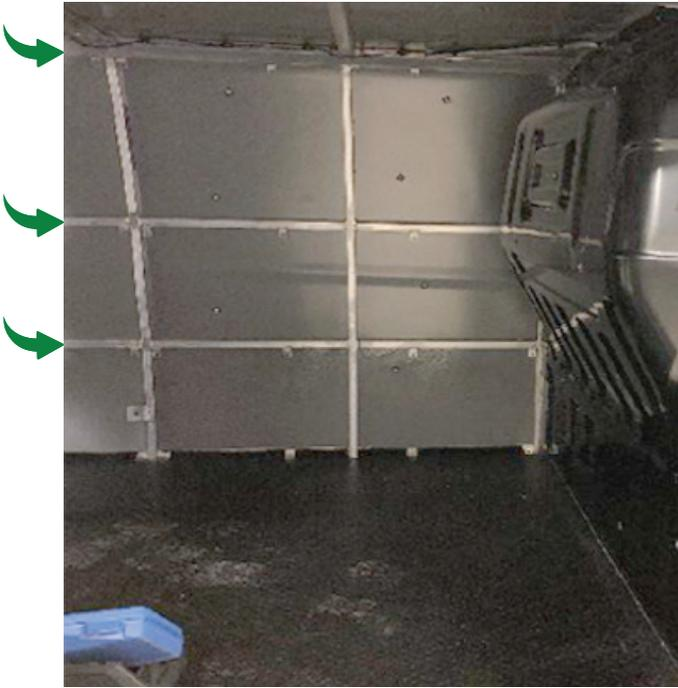
*The Modul-Rail are glued to the three thin horizontal beams of the vehicle*
