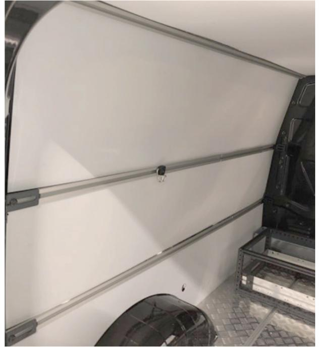
*Modul-Rail installed in vehicle.*
