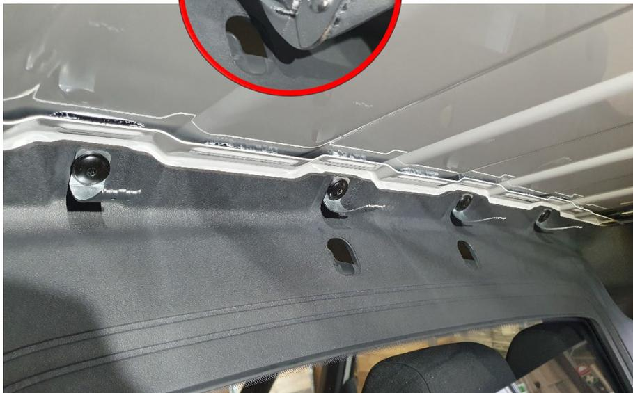
Fasten the roof lining board with lining screws as shown below.
