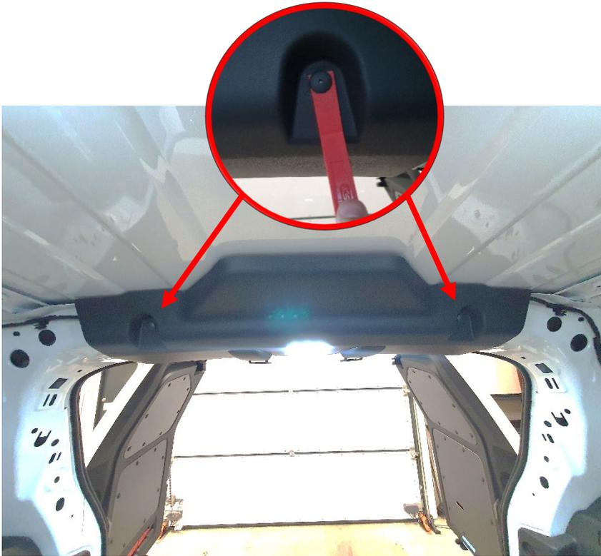
Install brackets (57110-03) in the same position using the original clips.
