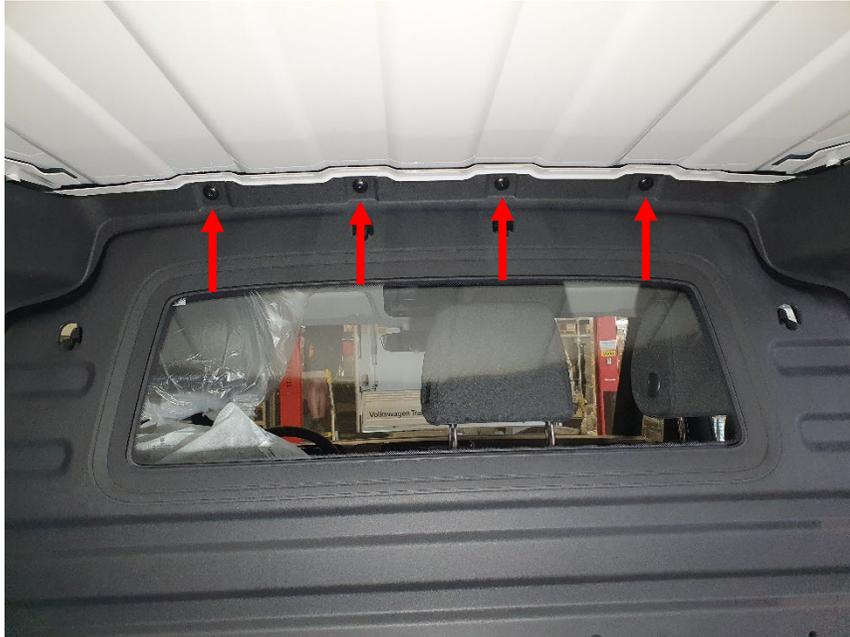
Install brackets (57110-03) in the same positions angled downwards using the original bulkhead screws. Ensure the screw is seated properly in the hole.
