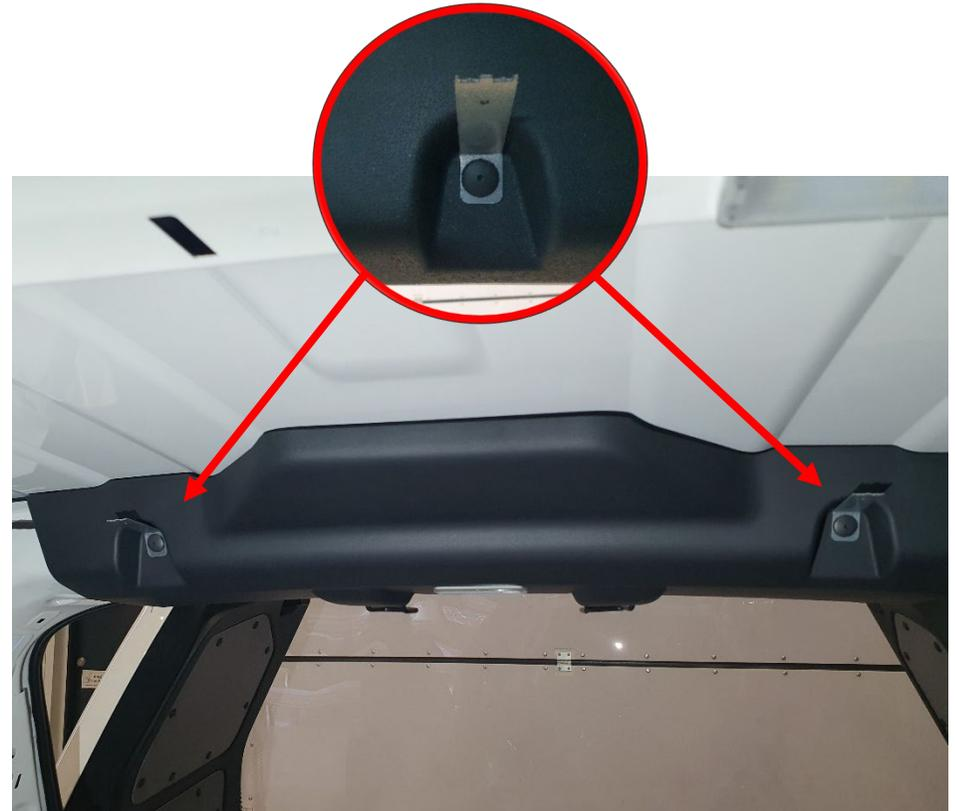
Remove the 4 screws in the top of the bulkhead.
