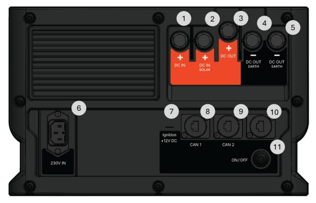
The CAN ports (number 8 and 9) in the rear of the units are for connecting the units.
