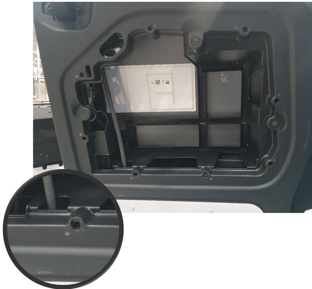
Screw with caution using the grey lining screw (p/n 36675-03 / 36677-03).
